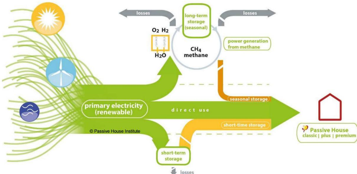
Figure 1-1 Energy flowchart from the RE supply to the energy consumed at the building, including facilities for short-term and seasonal storage. [3]
